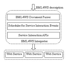
Fig. 5. Architecture of BML4WS interpreter.
